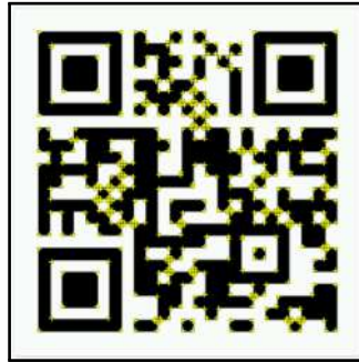
Figure 3.4 Tracking point given by Vuforia's algorithm
