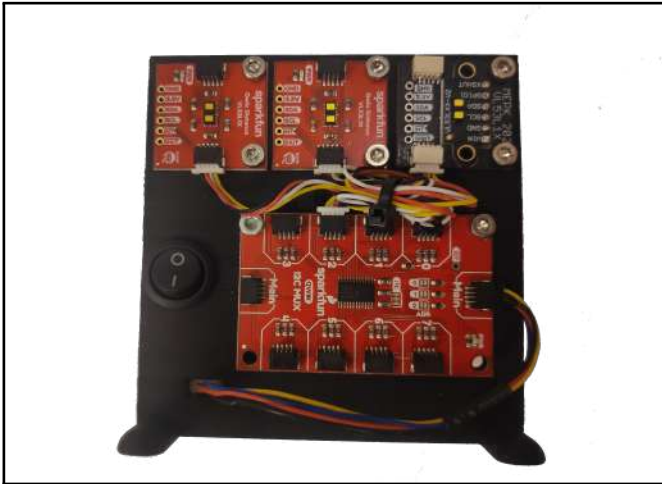
Figure 3.18 Set of three VL53L1X integrated with D1 mini Pro v2.0
