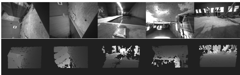
Figure 3.2 Stitched grey-scale image and corresponding depth map.
