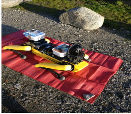
Figure 4.2 The two GPS systems mounted on Spot.
