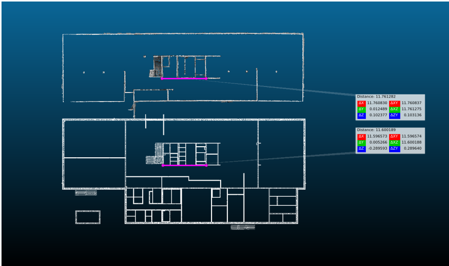
Figure B.3 Measured distance in reconstruction and BIM.
