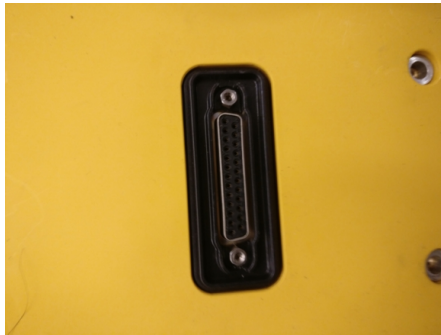
Figure 3.8 One of the two DB12 ports on Spot which provide the payloads with power and access to the internal network.
