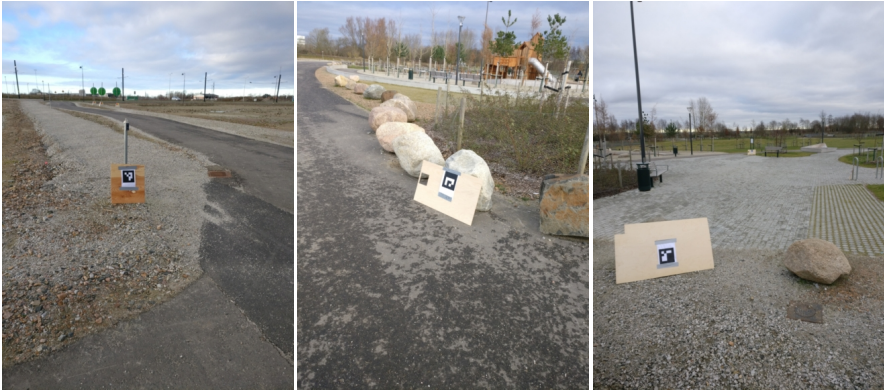
Figure 4.3 Placement of the fiducials during the localization experiments.
