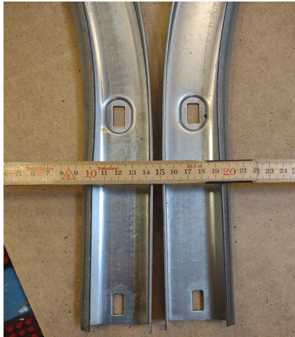
Figure 6.2: The inaccuracy in current bend-ends. The width of the bend-end on the left is 43mm and the one on the right 45 mm. According to schematics for the bend the width tolerance is supposed to be 42.3(+0/+0.7) mm.
