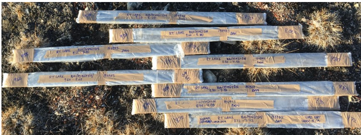
Fig. 4. The eight cores obtained with a Russian corer, which overlap according to how they are placed in the picture.
