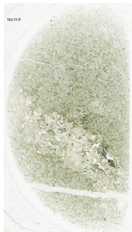
Figure A1. Thin sections showing suevitic impact breccia with chloritized rock fragments (H22-B08 C), suevitic impact breccia with kink bands in biotite (161.30 A), suevitic impact breccia (162.43) and clast-poor impact melt with calcite filled fractures (162.15 B).
