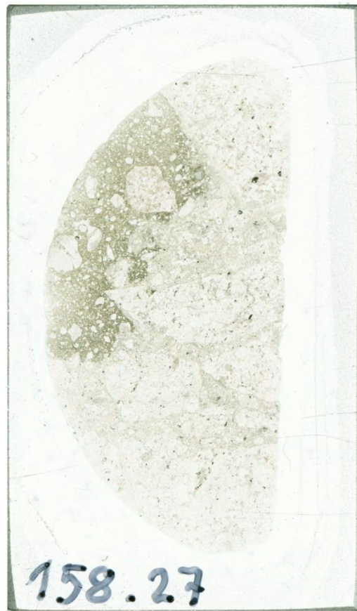
Figure A3. Thin sections from the field samples and the Hummeln-1 drill core. H22-F06:2) Suevitic impact breccia. H22-F06:3) Clasts of claystone displaying chloritized crystals. 160.68) sand-rich impact melt. 158.27) Suevitic impact breccia, the dark area contains clay and rounded quartz-grains with PFs.
