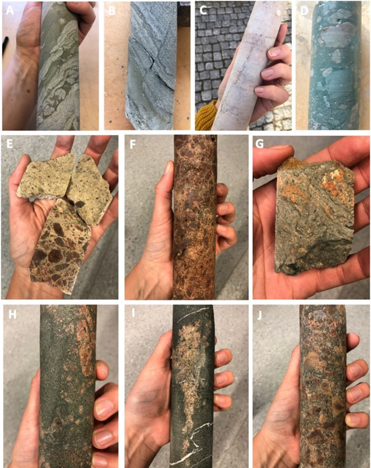
Figure 16. Photos of representative sections of the Hummeln-1 drill core in hand sample, the top of the stratigraphy is pointing upwards in all photos. A. Slump structures in a sandy mudstone (85.20 m). B. Faulting in sandstone interlayered with mudstone (80.10 m). C. Stylolite in carbonate rock (45.50 m). D. Carbonate breccia (48.15 m). E. Transition from breccia to arkosic sandstone (157.25 m, see Fig. 17). F. Monomict clast supported granite breccia 159.50 m. G. Sand-rich matrix with flow-structures (160.70 m). H. Polymict matrix supported breccia 161.20 m. I. Dark and fine-grained rock with granite fragments and calcite filled fractures (162.00 m). J. Monomict clast supported breccia with clay in matrix (164.10 m).
