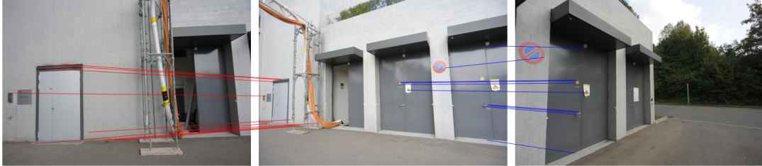
Figure 3.2 Single-view lifting allows next-view registration even with no three-view overlap between images. This omission in COLMAP limits it to only be able to register two views and one set of scene points (either red or blue).
