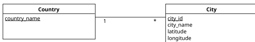
Figure 2.1: Relational database presenting the relationship between cities and countries. The underlined id:s are primary keys.
