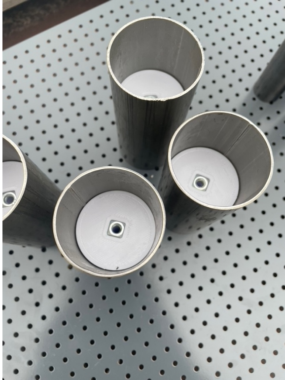
The \varnothing 50\text{mm} obstacles before being installed
