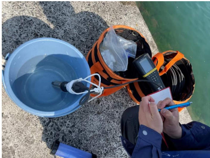
Fig. 2.6 Photograph of measuring water temperature and salinity (May, 2025)
