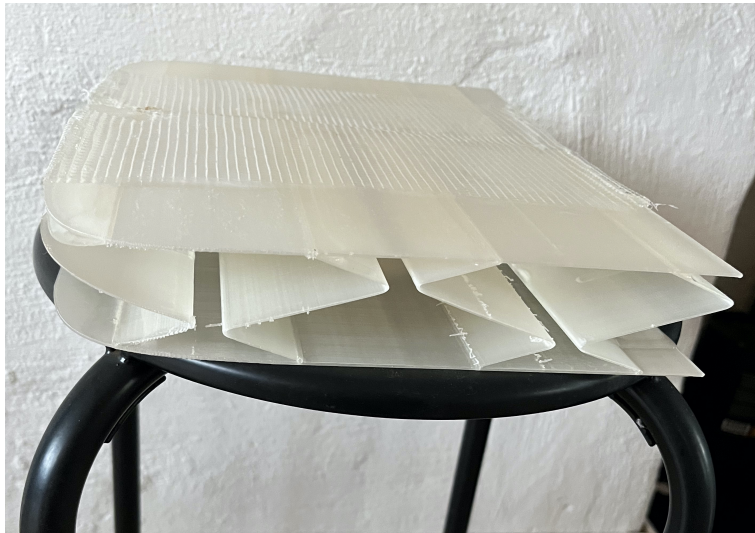
Figure 29: A printed prototype of a seat-cushion fused together in fiberglass.
