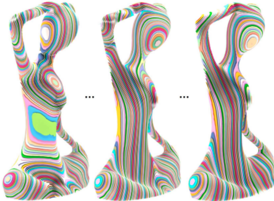
Figure 10: Three different slicings depending on print direction.[30]
