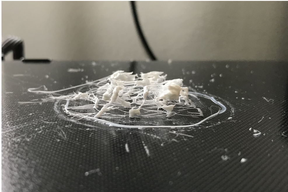
Figure 18: Failed print due to flexing struts.
