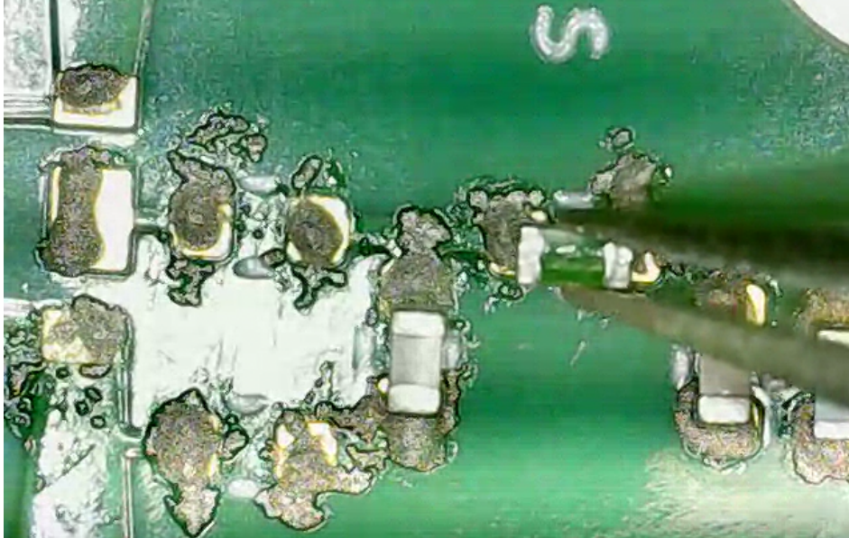
Figure 3.15: Microscope view when placing components on pads in solder paste
