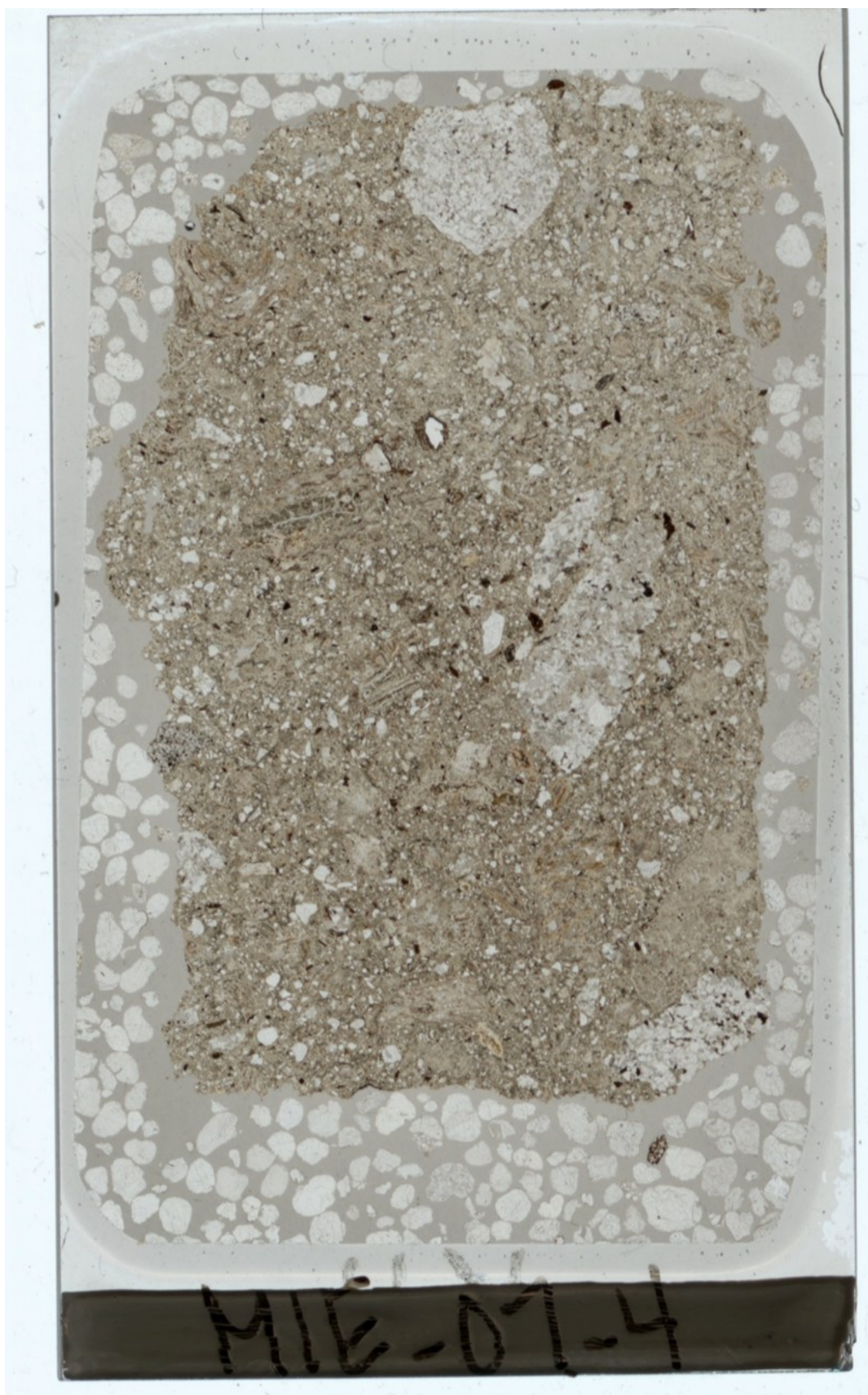
Appendix 1. One of six thin sections cut from the sampled impactites at Mien, which, besides petrographical studies with a compound microscope, were examined with SEM. MIE-M07-4 is a suevitic breccia type 2.
