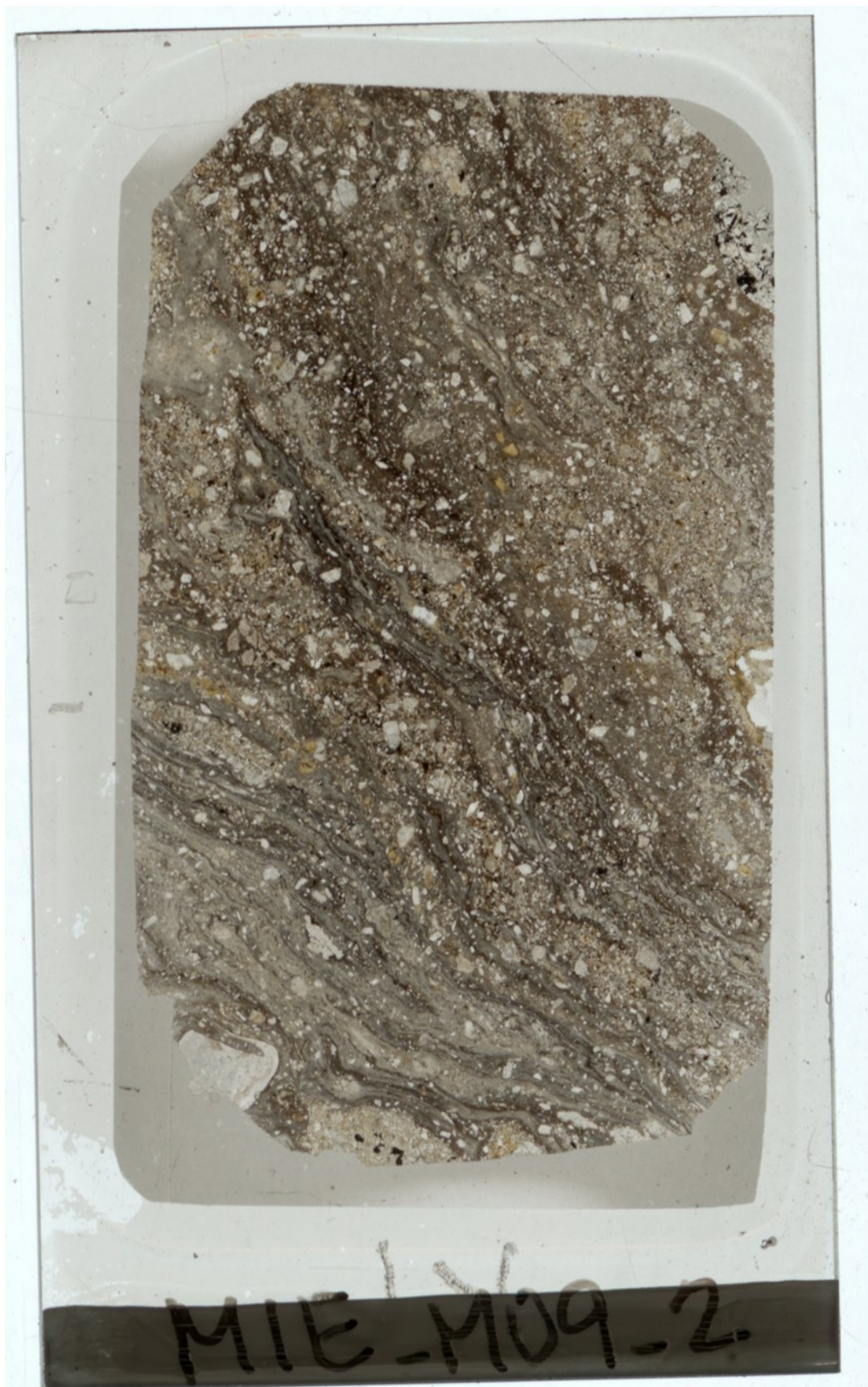
Appendix 2. One of six thin sections cut from the sampled impactites at Mien, which, besides petrographical studies with a compound microscope, were examined with SEM. MIE-M09-2 is an impact melt rock type 3.
