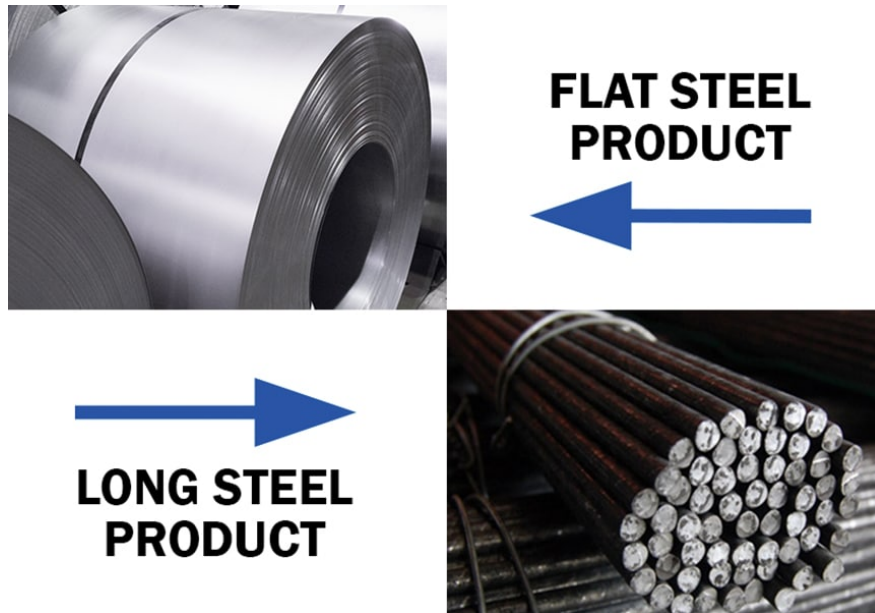
Figure 2: Long vs flat steel products (Sheffield Metals, 2018).
