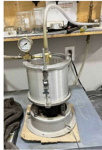
Figure 5. Vacuum apparatus connected to an agitation device.
