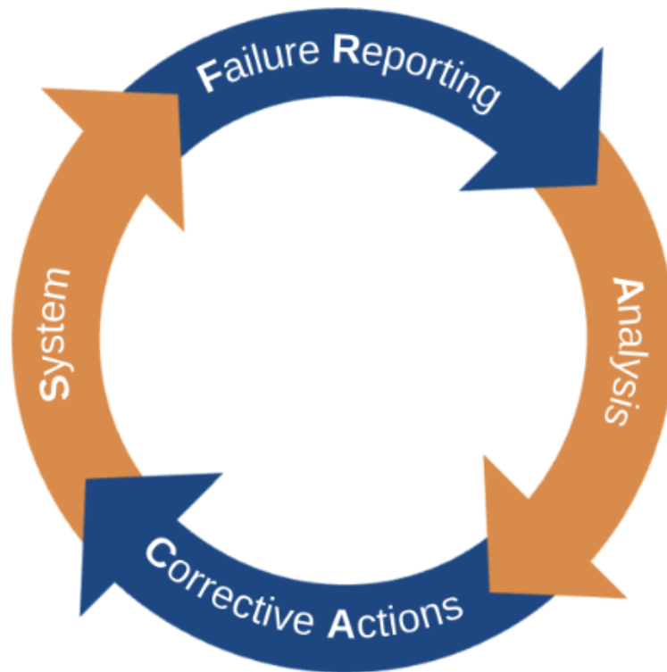
Figure 3.4: Illustration of the FRACAS closed-loop process.
