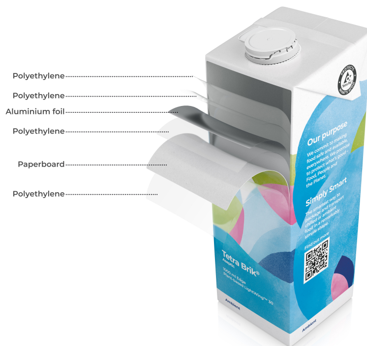
Figure 2.8: Anatomy of an ambient Tetra Pak packaging material. [9]
