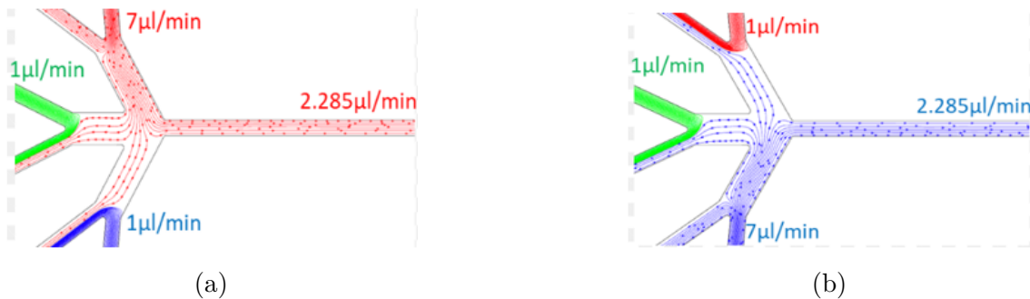
Figure IV.4: Simulation of microfluidic channels modulation. (a) With red color PBS flowing through the imaging region, corresponding to the “off” state. (b) With blue color fluorescein flowing through the imaging region, corresponding to the “on” state.
