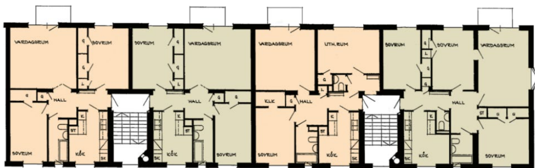
Figure 2: Floor plans of 1940s laminated timber houses. Source: Stockholms läns museum (n.d.), based on Tidstypiskt (2022).
