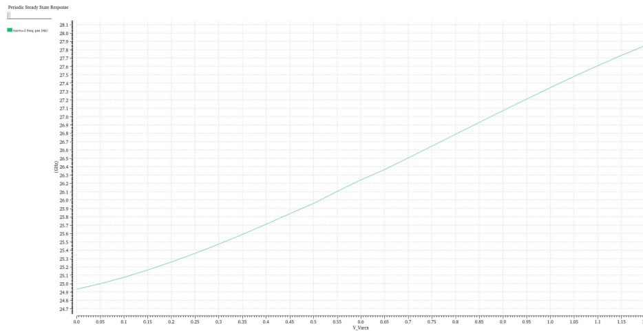
Figure 5.10: Combined tuning range of VCO and ILFD
