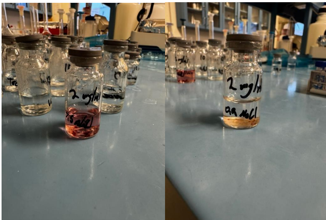
Figure 5.4. Visual instability in NaCl-containing CGRP 8-37 samples after storage. The 0.5% NaCl sample developed a pink color and gel-like spherical material, the 0.9% NaCl sample showed weaker but similar visible changes.
