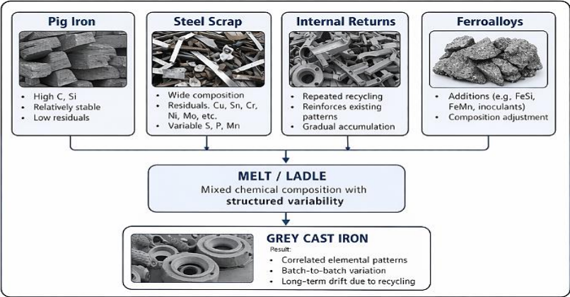
Figure 1. Flow of Material inputs and their characteristics, leading to structured compositional variability in the melt and final cast iron
