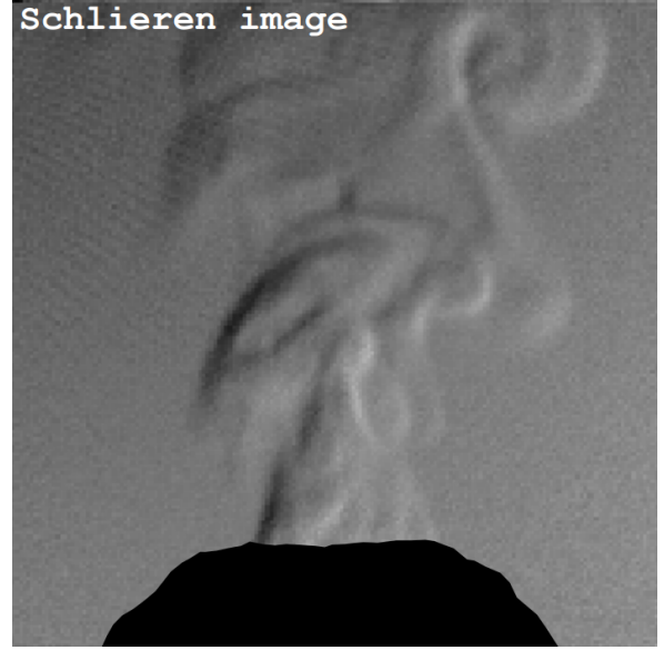
(c) The final gradient map generated by the software, visualizing the physical deflection of light caused by the heat from the candle.
