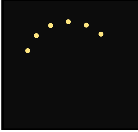
Figure 8: The spatial filter mask configured in the Fourier plane to select two independent triads of beams (six beams total) while blocking the remaining diffraction orders.
