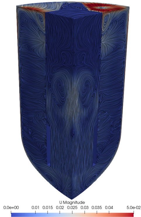
Figure 14: Velocity field in Boussinesq simulation under steady-state natural convection conditions.
