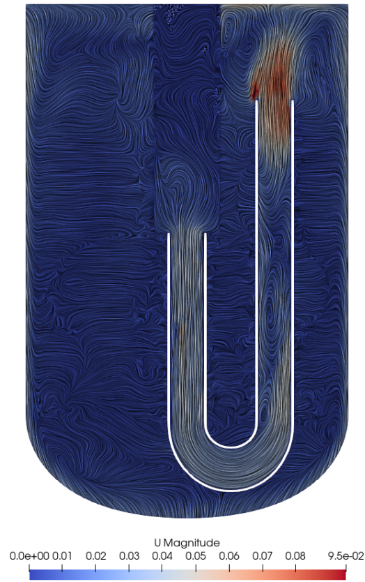
Figure 25: Velocity field in a vertical cross-section for the Boussinesq model.
