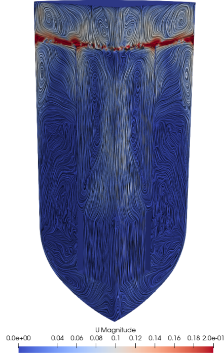
Figure 16: Velocity field in the VOF simulation under steady-state natural convection conditions.
