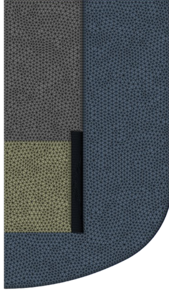
Figure 7: Forced convection mesh with cell size 0.05 m
