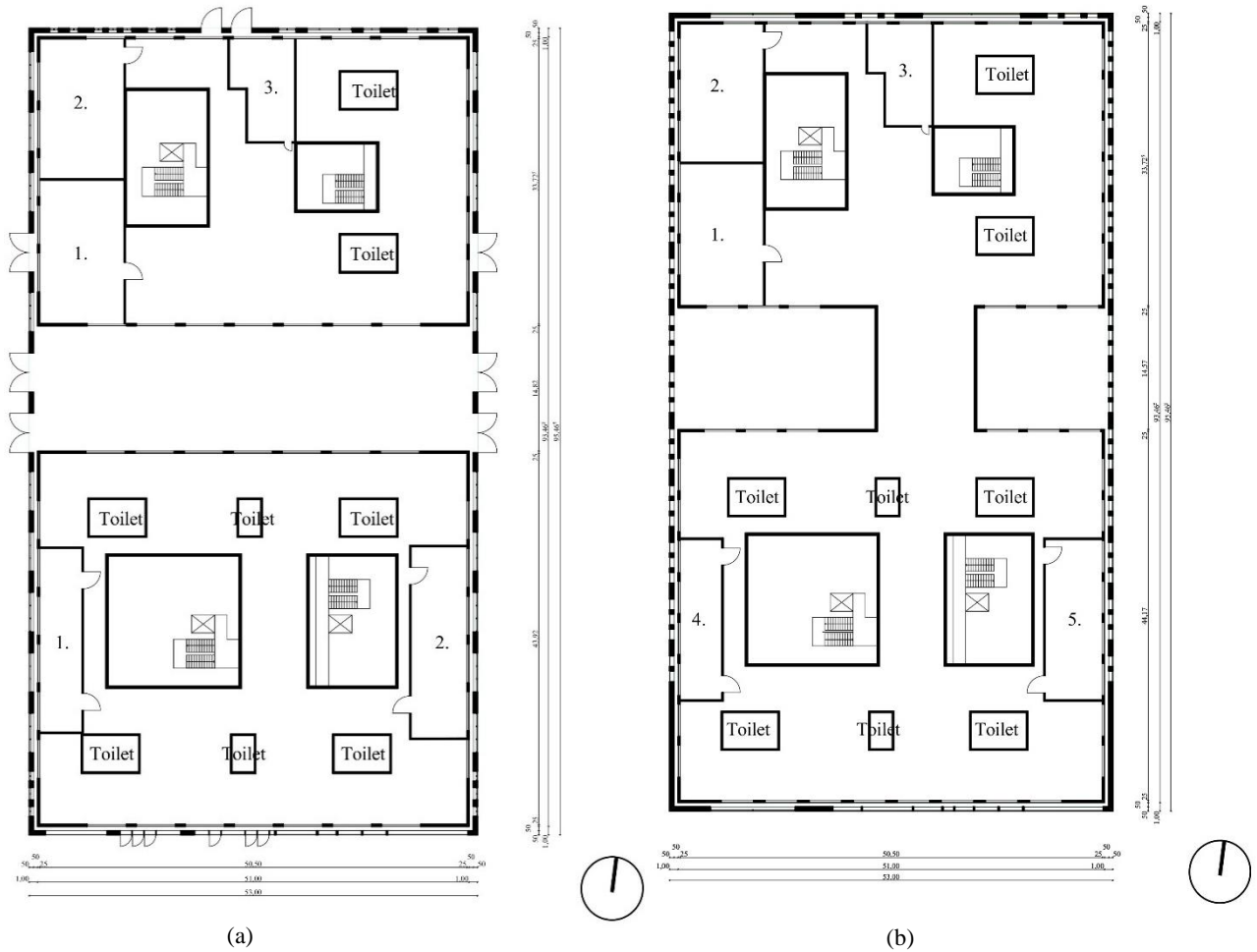
Figure 21 (a), (b) Educational program layout in 1:500 (left: ground floor, right: first floor)
