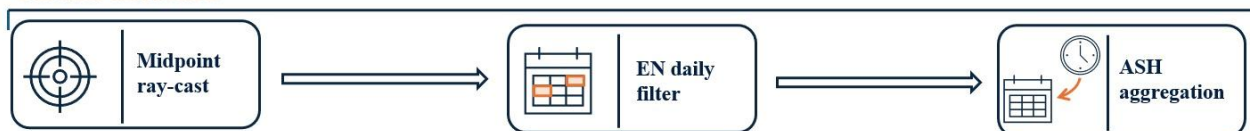
Figure 6 Workflow of the custom Grasshopper Python script used to calculate aperture-based and point-based sunlight access indicators.
