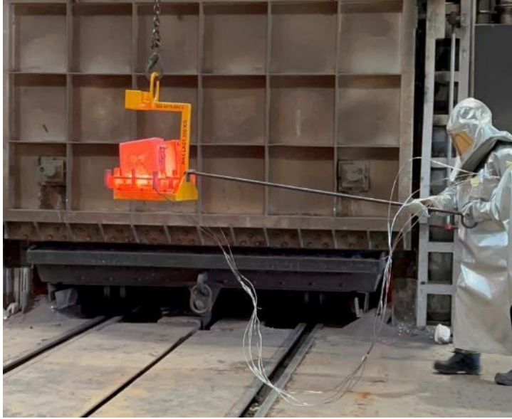
Figure 30: Moving the blocks to the quenching pool.
