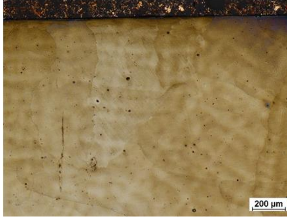
Figure 11: Dendritic structure in Hadfield Steel [8].
