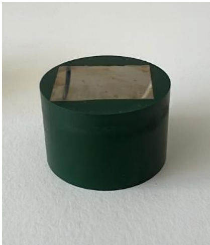
Figure 24: Example of a hot-mounted specimen.
