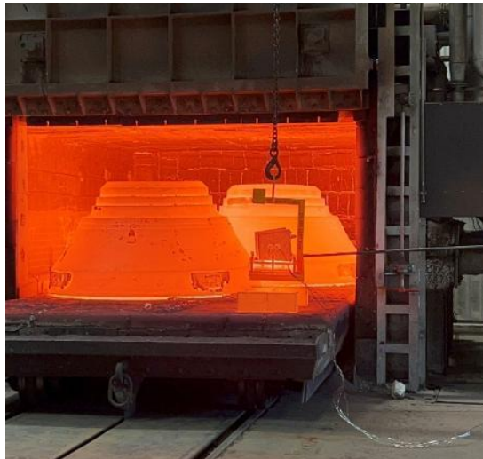
Figure 28: Taking out the blocks from the furnace.
