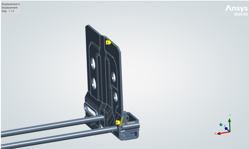
Figure 3.26: Illustrating of the boundary conditions used to constrain the model in the x-direction at Point A and in the z-direction at Point B.
