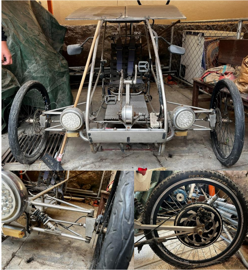
Figure 3-6. Images of the solar car: front suspension and the rear wheel motor (Source: Author).
