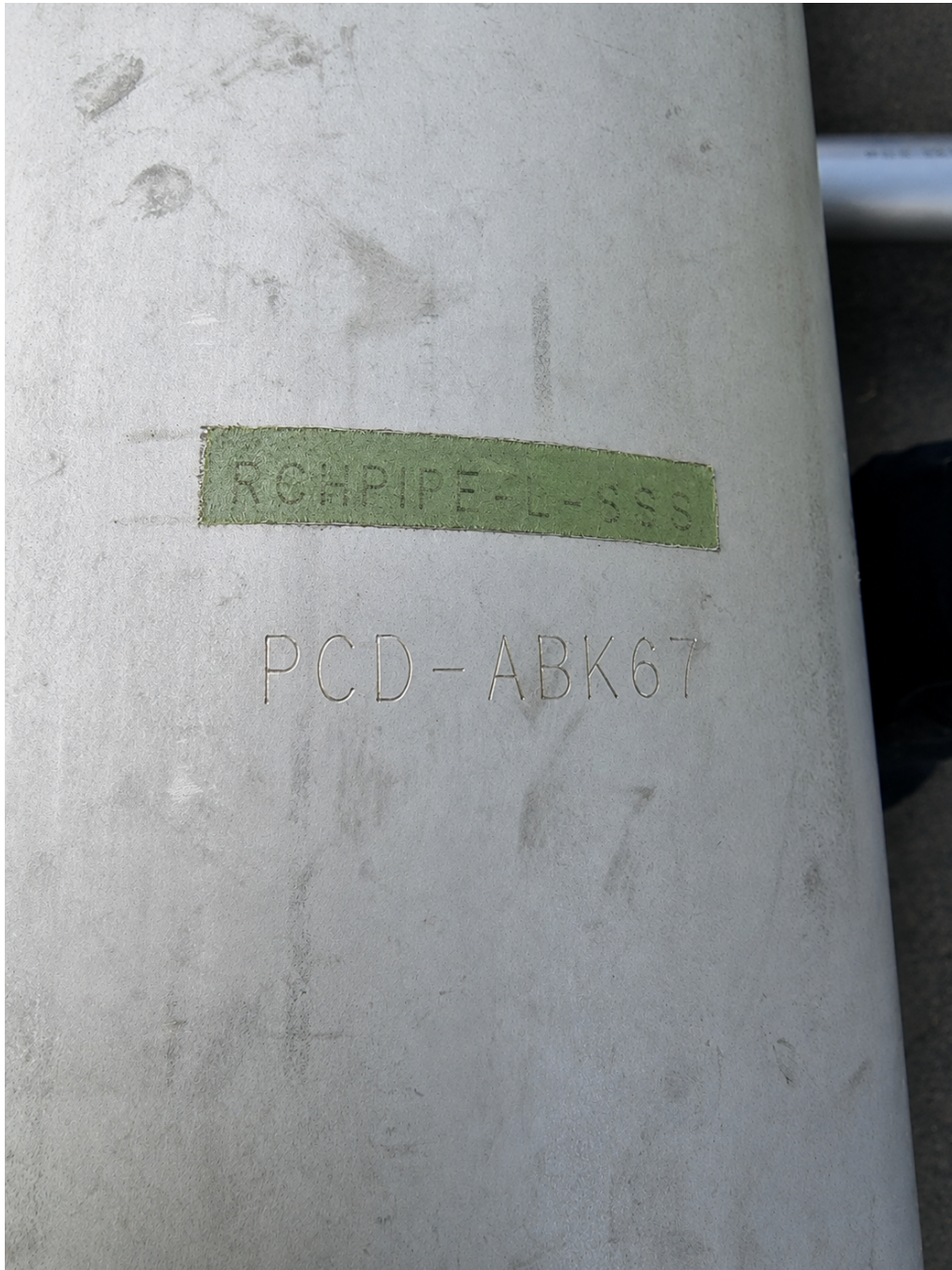
Figure B.5: Example of temporary markings affected by handling, production operations, or finishing processes.
