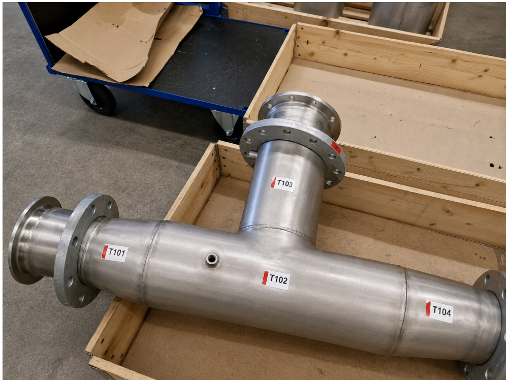
Figure B.4: Example of welding where multiple material identities become one physical assembly.
