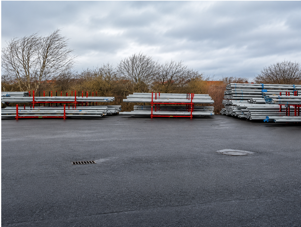
Figure B.1: Example of warehouse storage where pipes are grouped mainly by material type and dimensions.
