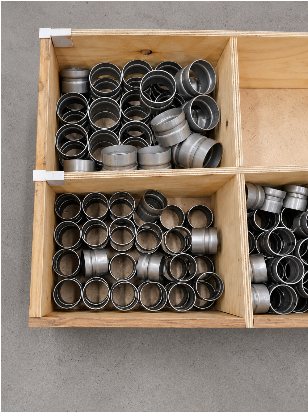
Figure B.2: Example of material grouped for production through crates, carts, and project separation.
