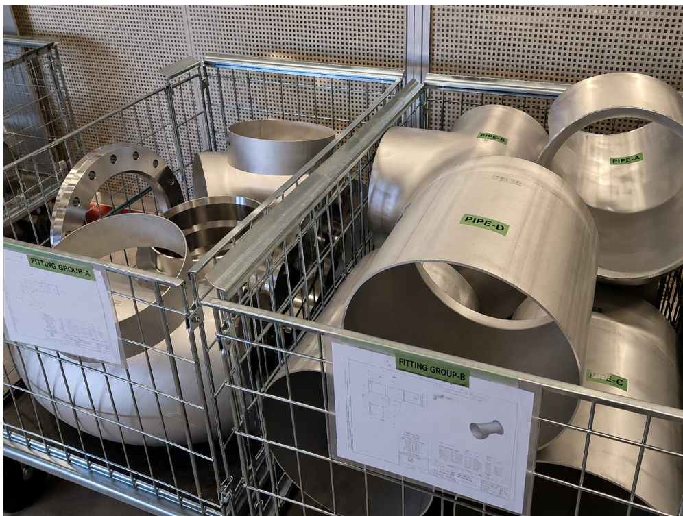
Figure B.6: Crates and carts used to maintain grouping during production flow.
