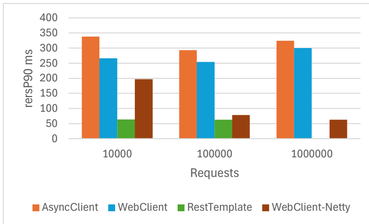
Fig. 28. Chart of response time in the 90 th percentile by number of requests sent
