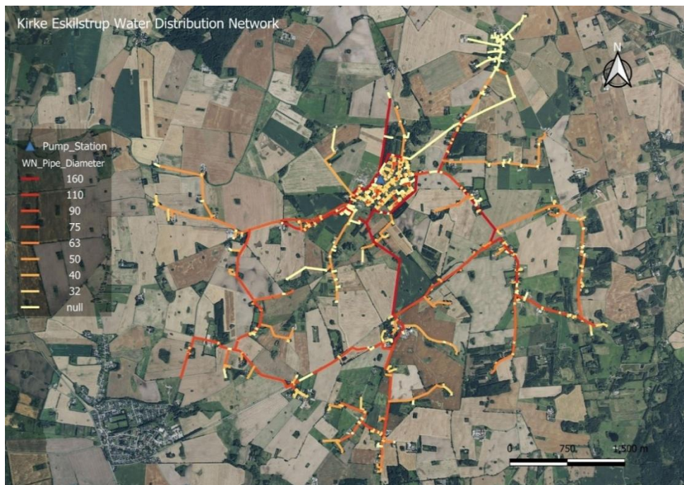
Figure 4.4. Distribution of Pipe Diameters
