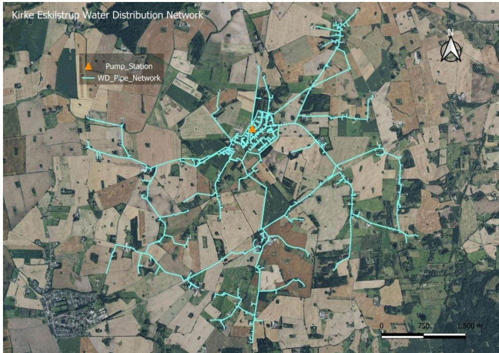
Figure 4.3. Kirke Eskilstrup Distribution Network
