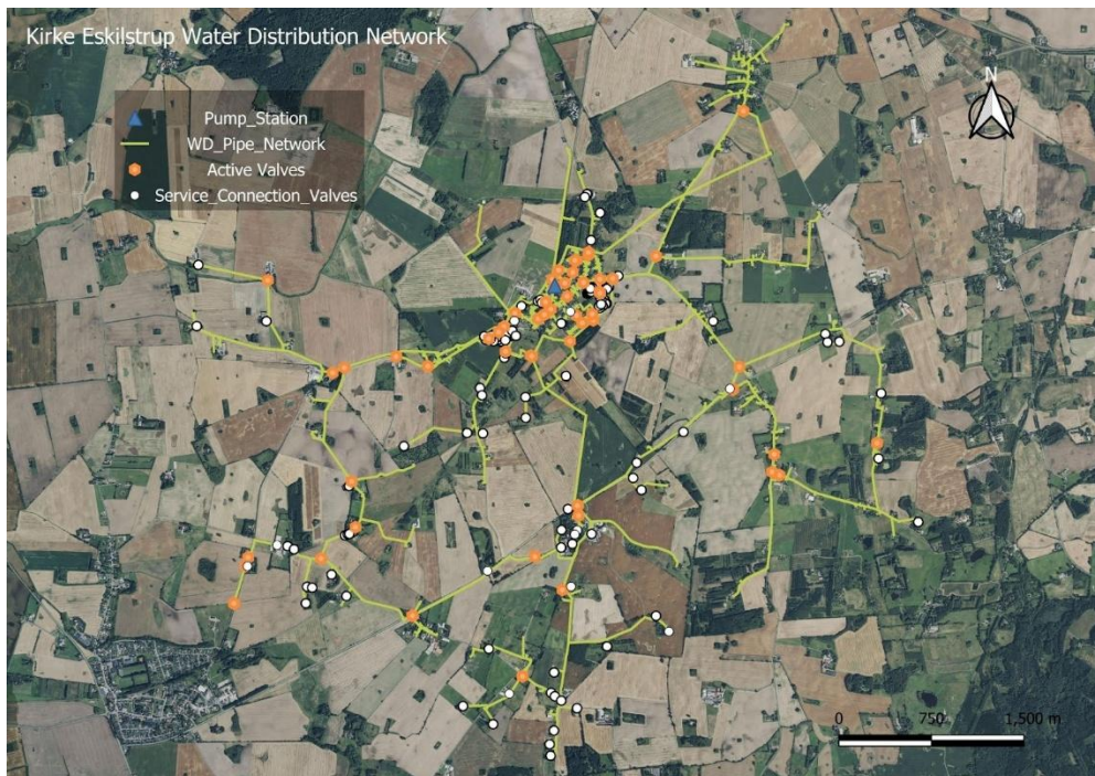
Figure 4.6. Valves within the Water Network
