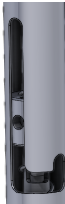
Figure 42: The L-slot with the solo-runner inside
