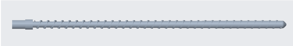
Figure 6.20: Optimized screw geometry for targeted mass flow rate (medium volume) and minimized power consumption.
