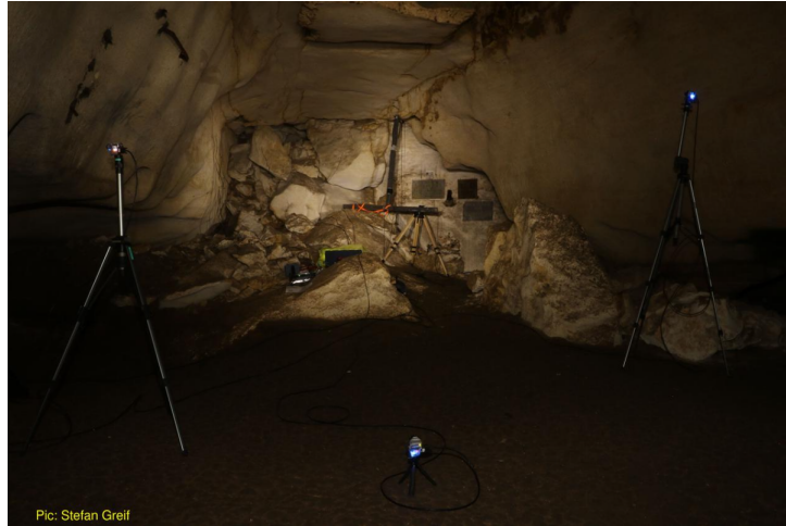
Figure 5: The experimental set up in the Orlova Chuka cave. The black inverted T in the center of the image holds four microphones. Six smaller microphones are mounted on the left wall and not visible in this photograph.
