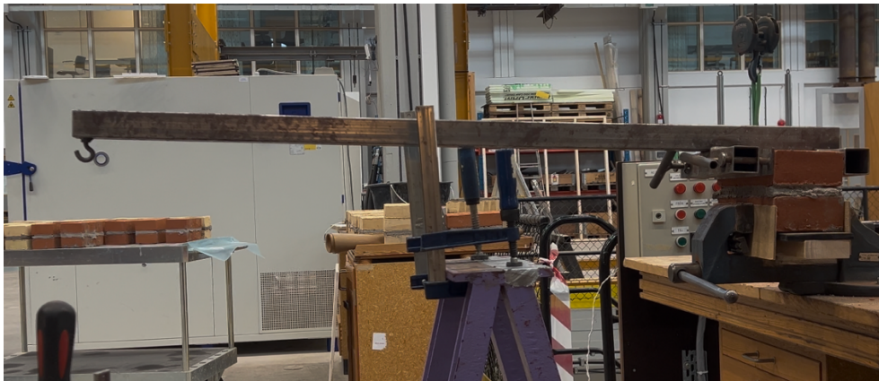
Figure 9: Bond wrench setup used in this study. The purple stand located at the centre of the figure was installed as a safety measure. In the event of specimen failure, the lever arm may become detached and fall; therefore, the stand acts as a barrier to prevent the lever arm from falling.
