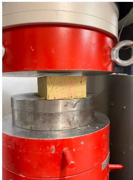
Figure 3: Brick unit in cube press to determine compressive strength capacity of brick.
