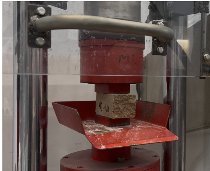
Figure 5: Compression strength testing of mortar prisms.
