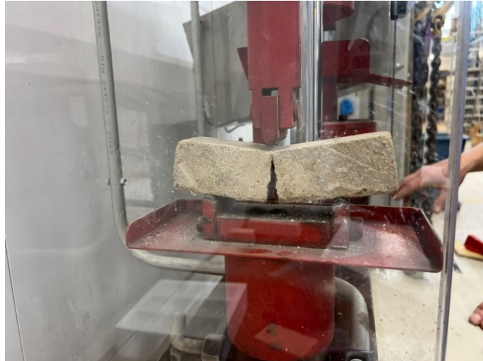
Figure 4: Flexural capacity test of mortar prism.
