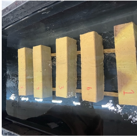
Figure 1: 24h absorption test of bricks where ten bricks were put into water buckets for 24 hours after drying at 105 °C.
