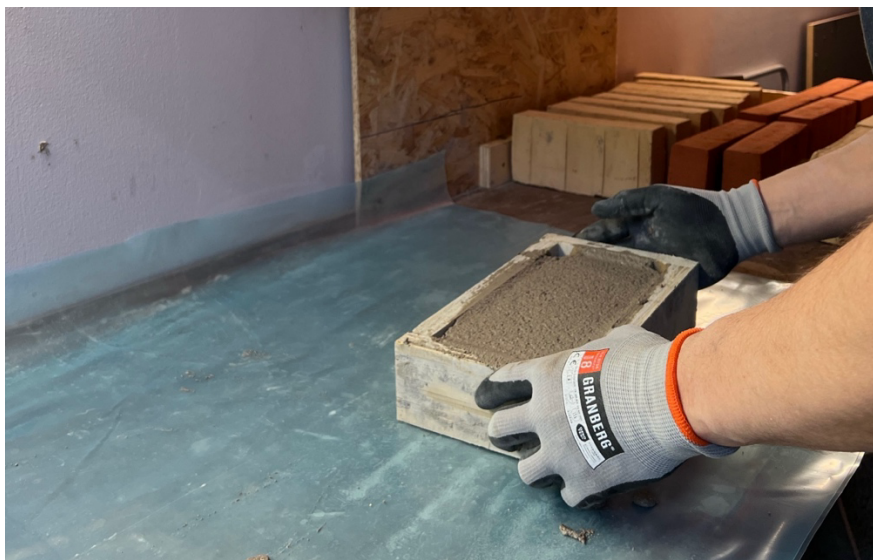
Figure 6: Preparation of masonry couplet specimens using a timber mould to control bed joint thickness.
