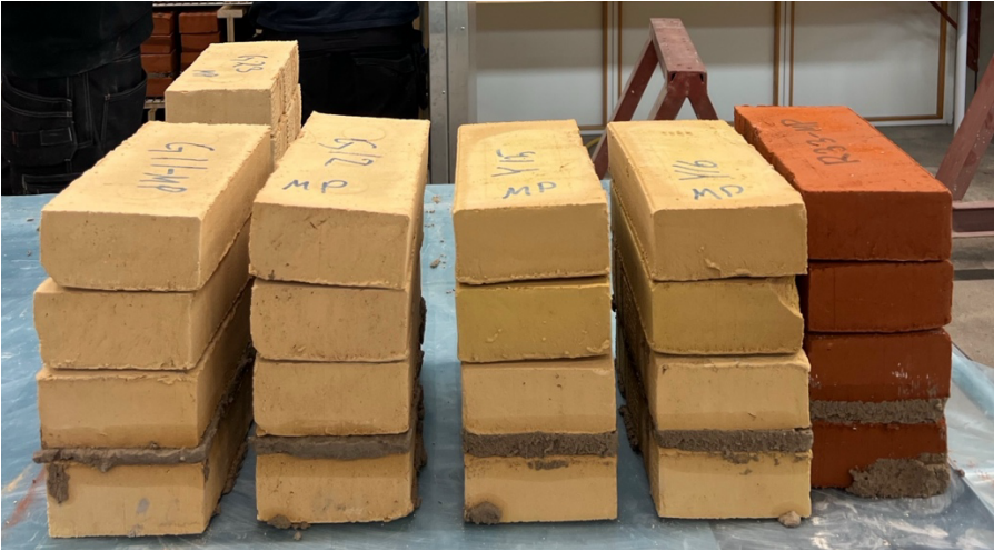
Figure 7: After Specimens are assembled, two bricks are added onto the top to create pressure of approximately 2 \times 10^{-3} \text{ MPa} for the curing process.
