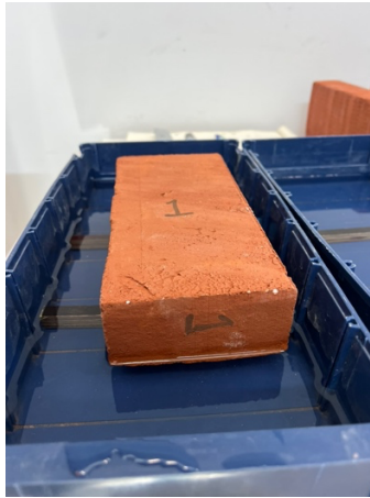
Figure 2: Brick in water of a depth of 3-5mm for water absorption coefficient determination.
