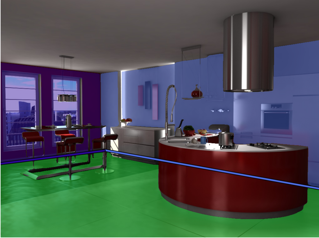
Figure 5.2 Floor-wall intersection lines, ai_001_005/c0/f0 (floor 0.964, wall 0.764, ViT-L + Swin-Large). Each coloured line segment shows the 3D intersection of a detected wall plane with the detected floor plane, projected back to the image plane. Wall and floor masks are shown as coloured overlays, and the intersection line for each wall uses the same colour as its mask.
