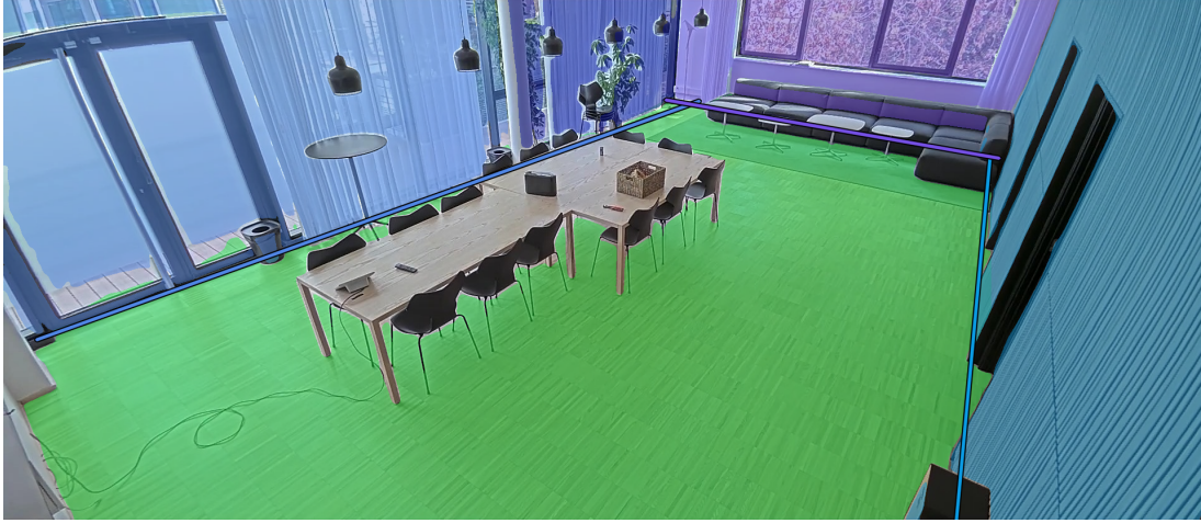
Figure 5.4 Floor-wall intersection lines, Lunch Room Corridor (floor 0.971, wall 0.880, ViT-L + Swin-Large). Each coloured line segment shows the 3D intersection of a detected wall plane with the detected floor plane, projected back to the image plane. Wall and floor masks are shown as coloured overlays, and the intersection line for each wall uses the same colour as its mask.
