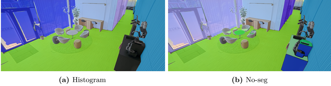
Figure 4.11 Coffee Lounge (ViT-L + Swin-Large). In the no-seg prediction, table tops and sofa seats satisfy the upward-normal floor condition and are predicted as floor alongside the true floor. Cabinet sides are predicted as wall.
