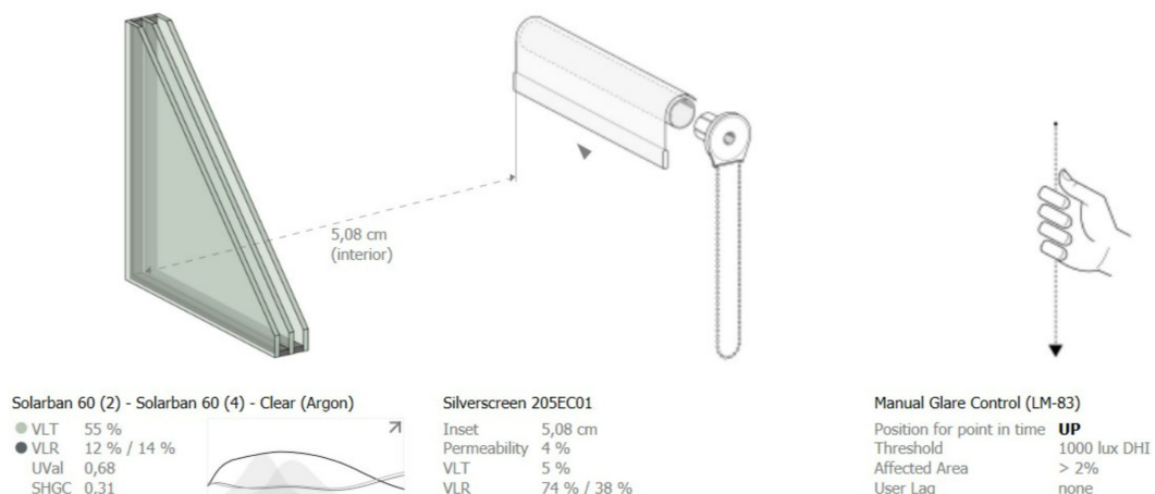
Figure 14. Glazing and shading properties assigned to the façade glazing in the base
