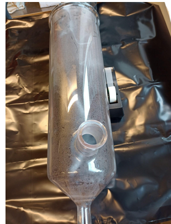
Fig 6: Photograph of the model after spray drying at 100% aspirator Flow height 45 mm Visible deposition is observed primarily in zone (right wall) and zone C (outlet tube)
