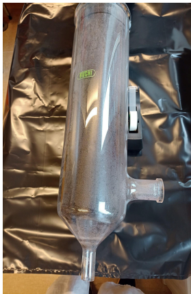
Fig 5: Photograph of the model after spray drying at 100% aspirator, flow height 60 mm. Deposition is visible in all zones, but with a different distribution compared to the 45 mm flow height case.
