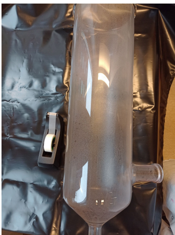
Fig 5: Photograph of the model after spray drying at 100% aspirator, flow height 60 mm. Deposition is visible in all zones, but with a different distribution compared to the 45 mm flow height case.
