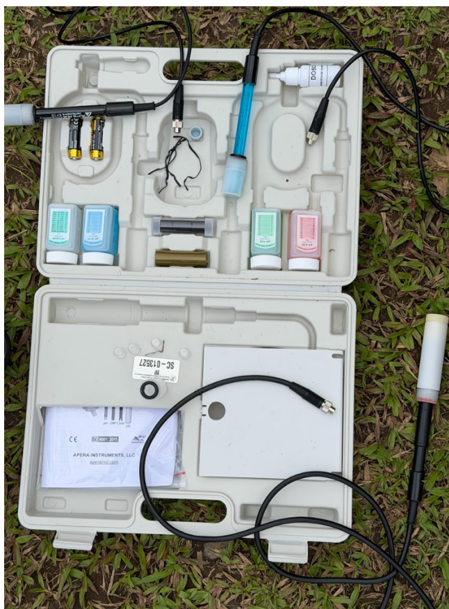
Figure 4.9: Portable multimeter probe (APERA SC751) used when measuring water quality.
