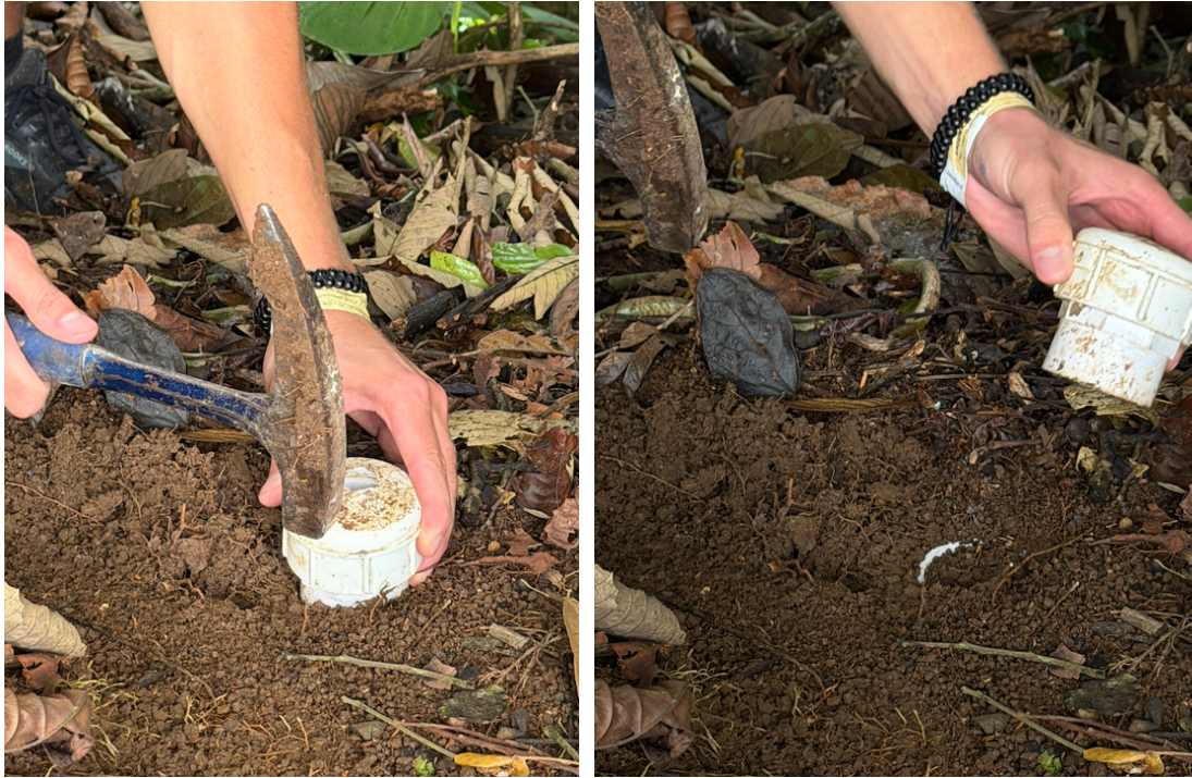
Figure 4.3 and Figure 4.4: Soil sampling by gently hammering down a PVC ring into the top layer of the soil. The right picture shows the ring when it has been hammered down into the soil.
