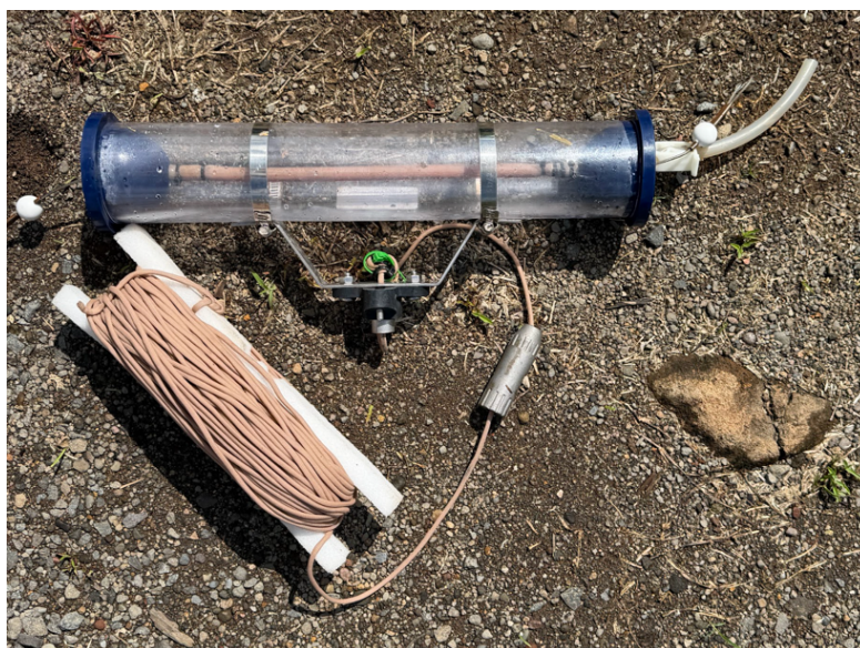
Figure 4.8: Kemmerer water sampler used for collecting water samples at selected depths in the water column.
