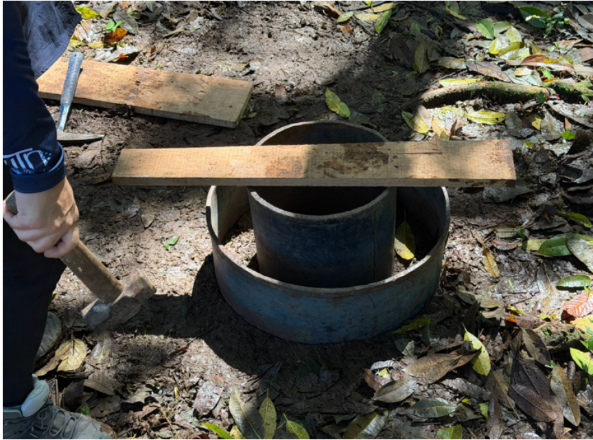
Figure 4.5: Double ring infiltrometer in field.
