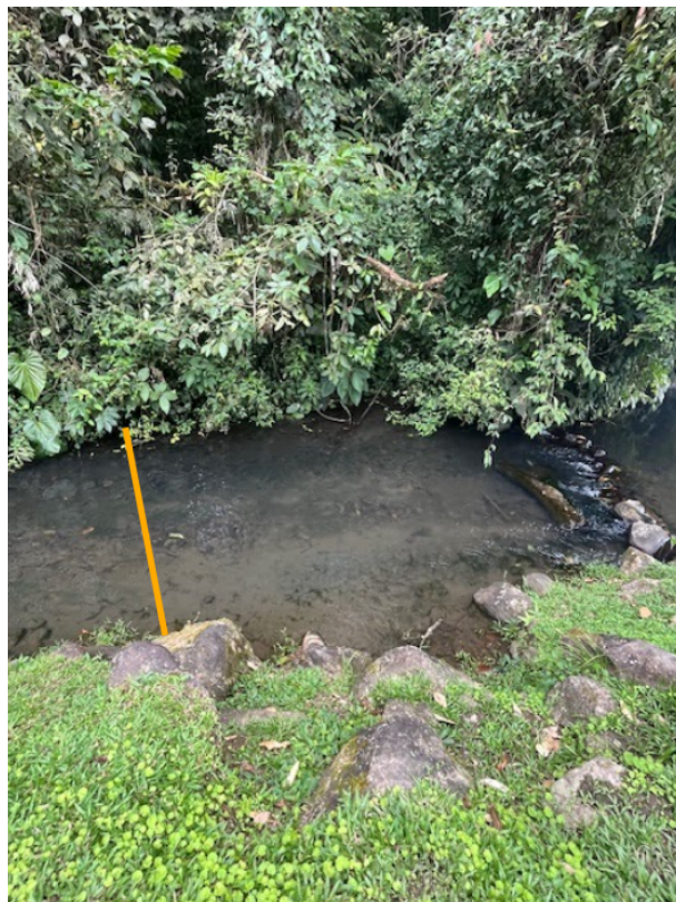
Figure 4.6: The only visible outflow from the lake. The figure shows water flowing east, left in the image. The orange line represents the 4.8 m wide cross-section used for flow measurements.
