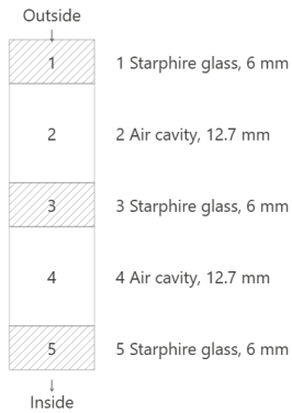
Figure 16: Layer assembly of CS library window.
