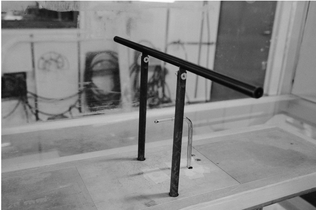
Figure 3.26 Pitot Tube Calibration with a 12 mm Cylinder Model Mounted
