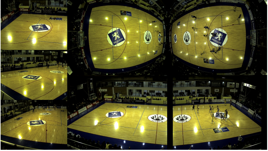
Figure 3.1 Overview of the APIDIS dataset multi-view framework. The dataset captures a full professional basketball game with a total duration of approximately 2 hours. The synchronized multi-camera setup consists of 7 calibrated viewpoints (including 5 lateral perspective color cameras and 2 overhead fisheye cameras) recording concurrently at an average frame rate of 22 fps and a native resolution of 1600 \times 1200 pixels. The panel illustrates synchronized frames across all active cameras at a single temporal anchor.
