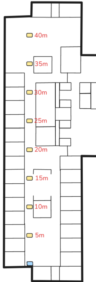
Figure 3.5: Line-of-sight test corridor with an unobstructed propagation path up to approximately 40 meters.
