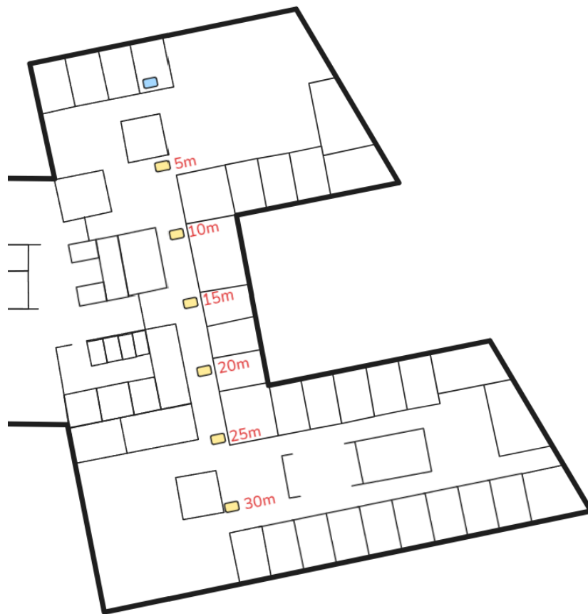
Figure 3.6: Non-line-of-sight test corridor where glass and drywall partitions obstruct the direct signal path.
