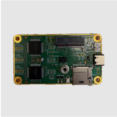
(a) Data unit based on ADS1299 chips for multi-channel EMG signal recording.
