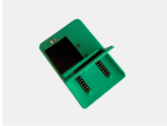
(b) Electrode interface module used to connect the flexible electrode array to the acquisition system.
