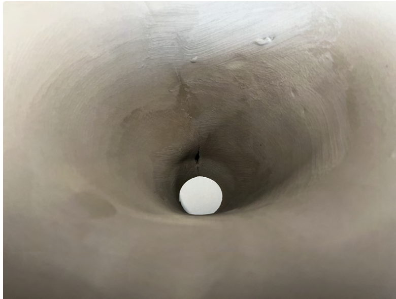
Figure 6.9: Crack at the throat of the initial OS attempt.
