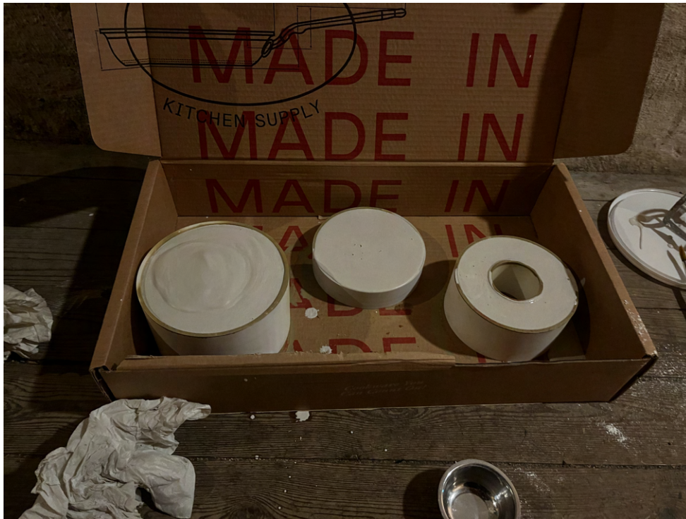
Figure 4.7: Initial failed attempt at casting plaster into a 3D-printed form.
