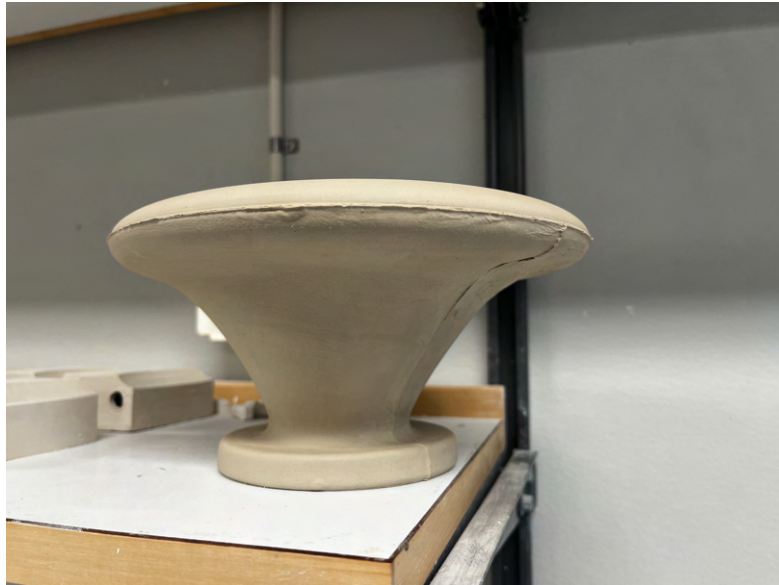
Figure 6.11: Seam lines present after demoulding.
