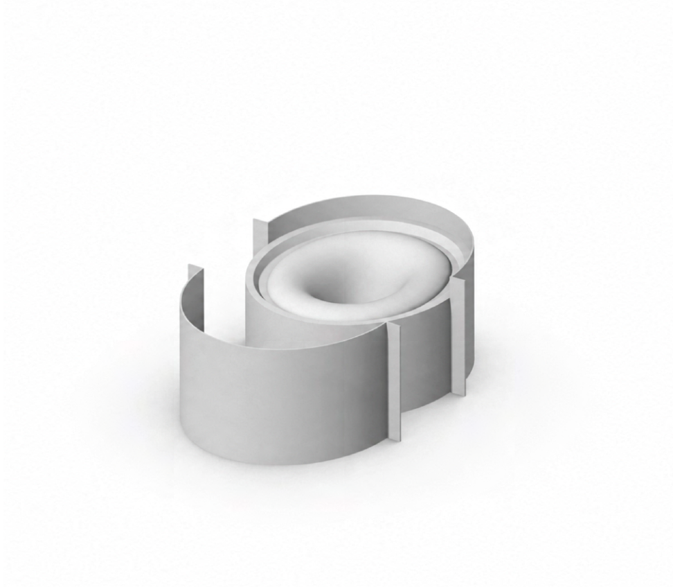
Figure 5.8: 3D printed mould positive showing face and fence
