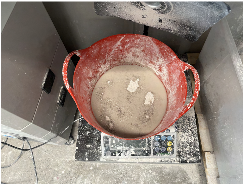
Figure B.1: Formation of “plaster islands” during mixing, indicating that the plaster-to-water ratio is approaching saturation.
