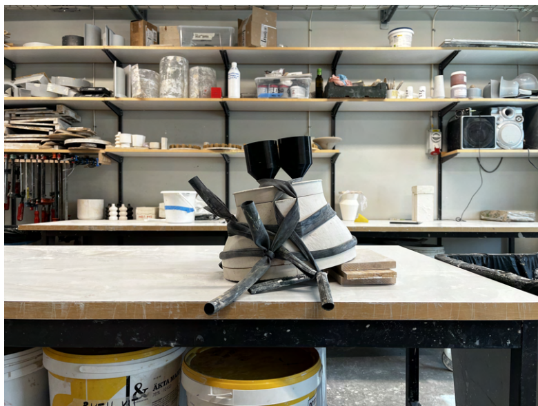
Figure 6.10: Improved mould setup for casting the OS horn.
