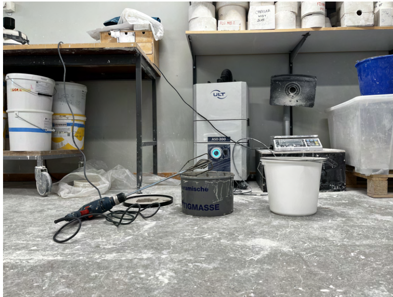
Figure 6.8: Mixing slip with a drill before straining it into a separate bucket.
