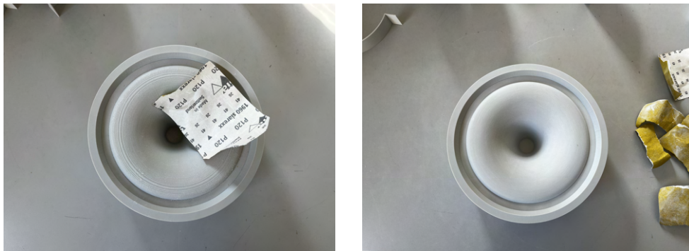
Figure 6.1: 3D printed surface positive before and after sanding.
