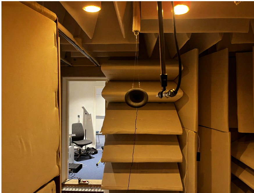
Figure 7.6: Front view of the measurement setup illustrating microphone alignment limitations.
