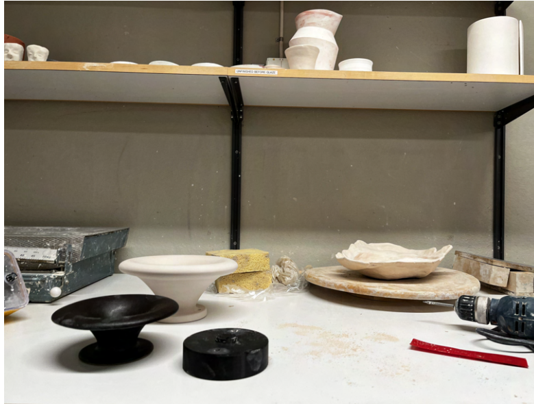
Figure 6.13: 3D printed drill template used for drilling bisqueware.
