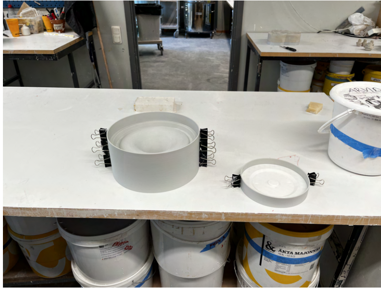
Figure 6.2: 3D printed mould positives assembled and ready for plaster casting.
