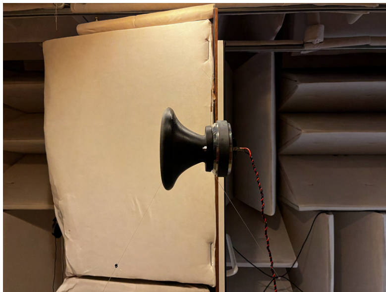
Figure 7.2: Side view of the suspended horn measurement setup.
