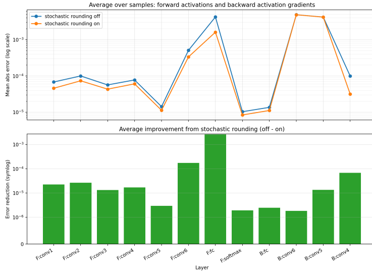
Figure 4.17: Layer-wise activation error comparison between RTL results and floating-point reference with and without stochastic rounding.
