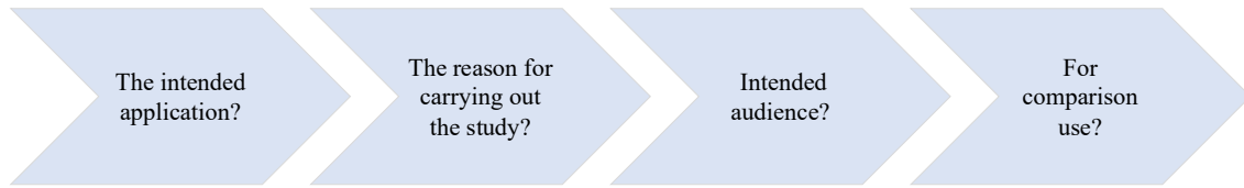
Figure 6. Goal definition requirements of the LCA study, adapted by the author from [53]
