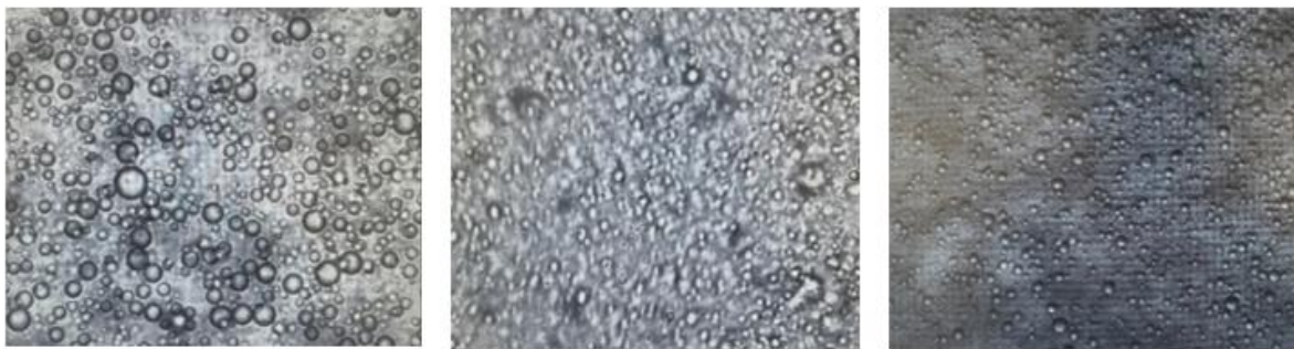
Figure 3. Microscope views of the a) non-homogenised sample, b) homogenised sample, c) sample treated with Ultra Turrax, respectively.
