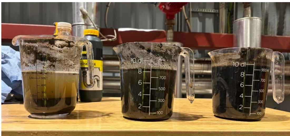
Figure 3: Results of the coagulation tests performed on the sieved digestate samples using \text{FeCl}_3 .
