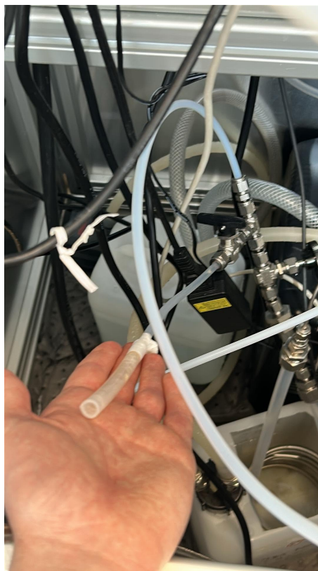
Figure 3: Silicone tube setup for the Dräger tubes to be inserted into
